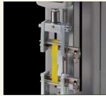
PP band tension strength test with PPC-5000N.
