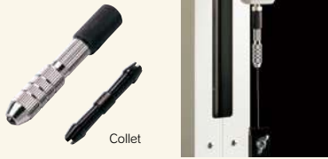
Wire tension strength test with CP-150N
