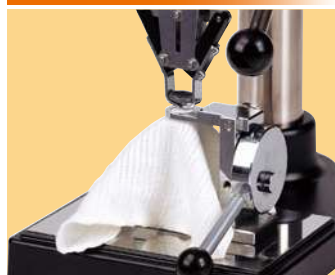
Cloth Button Pull Off Test
