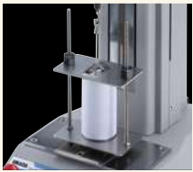
Opening testing for pull-tab of beverage can
