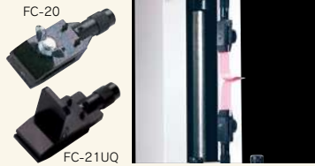
180 degree peel testing of adhesive tapes with FC-21
