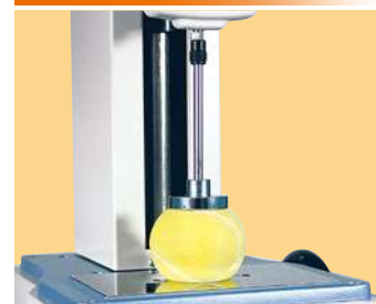
Ball Hardness Test
