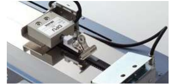
Peel test of embossed carrier tape
