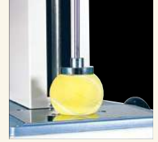
Ball compression test with S-40.
