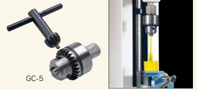
Resin molding tension exertion strength test with GC-5.
