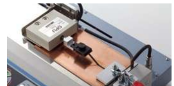
Peel test of copper foil
