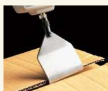
Corrugated card board opening strength test with DF-60
