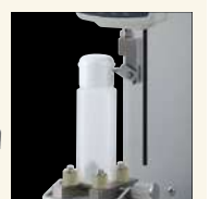
Flip Cap Opening test with HFC-50N
