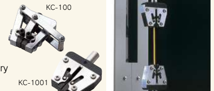
Cable tension strength test with KC-1001.
