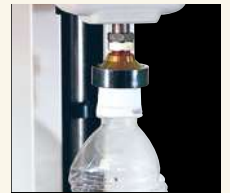
PET bottle compression strength test with PC-5060.
