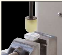
The switch tactile test with UR-8S.
