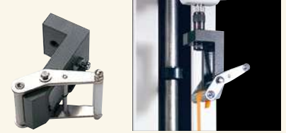
Rubber tape tension strength test with GC-60.
