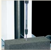
Sponge hardness test with PG-2.
