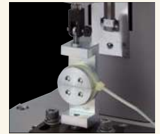
Binding band tension strength test with LOP-1000N
