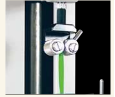
Rubber tube tension strength test with GP-15
