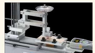
Coefficient of friction test for lipstick&artificial skin
