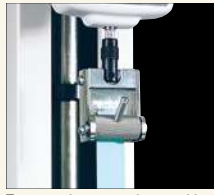
Tape tension strength test with GR-30.
