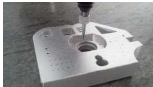
Needle contact-point mounting example
