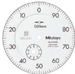
Graduation: 0.01 mm, Measuring range: 10 mm 29025
