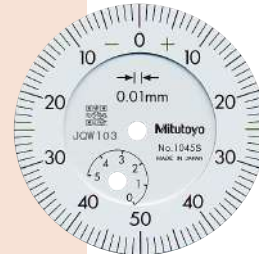
Graduation: 0.01 mm, Measuring range: 5 mm 10455
