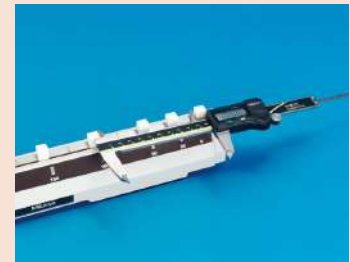
Checking accuracy of caliper (inside measurement)
