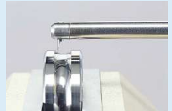
Inner/outer ring contour of a bearing
