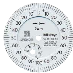
Graduation: 0.002 mm, Measuring range: 1 mm 10135-10 Shockproof Jeweled bearing
