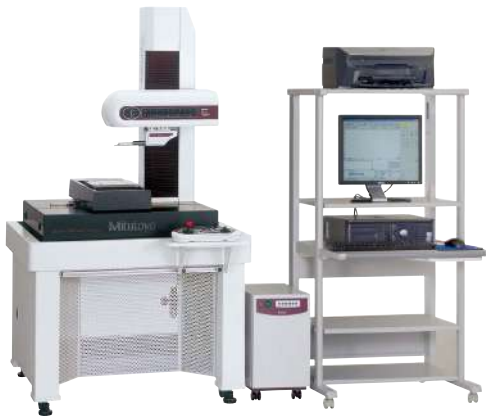
SV-3000CNC (Inclinable drive unit + Y-axis table)
