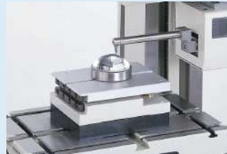
Aspheric lens contour
