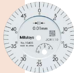
Graduation: 0.01 mm, Measuring range: 3.5 mm 10405 Double scale spacing
