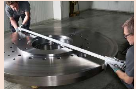
Radiused jaws for accurate ID measurement
