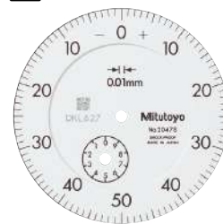
Graduation: 0.01 mm, Measuring range: 10 mm 20475
