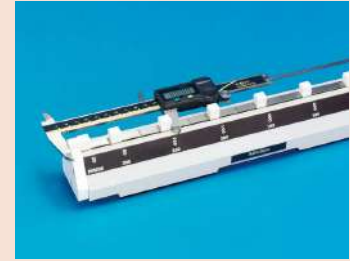
Checking accuracy of caliper (outside measurement)
