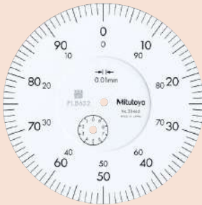
Graduation: 0.01 mm, Measuring range: 10 mm 3046S
