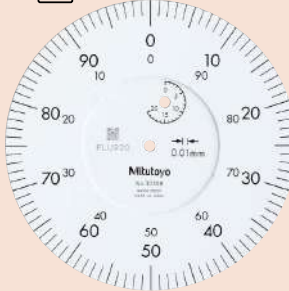
Graduation: 0.01 mm, Measuring range: 20 mm 3050S
