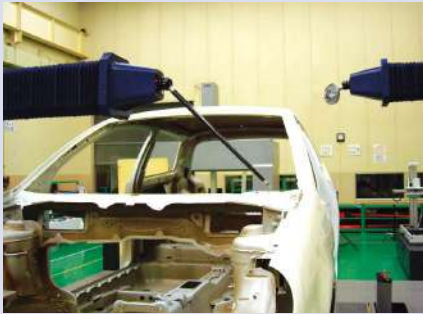
Measurement example for dual-ram type (Simultaneous use of touch-trigger probe and line laser probe)
