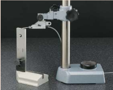
Setting a dial test indicator to a long-gauge-block stack attached to the base with a D-type connector
