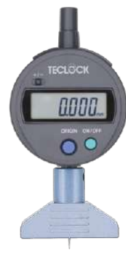
DMD-2500S2 Needle Contact Point Resolution 0.001mm Measuring Range 5mm
