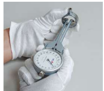
Measuring example of inner diameter of a small metal work piece.
