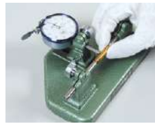
Measurement example for swing of round bar.
