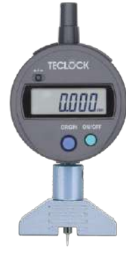
DMD-2520S2 φ3.2 Steel Ball Contact Point Resolution 0.001mm Measuring Range Concave 5mm Convex 4mm
