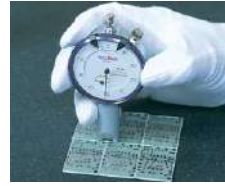
V-Grooved depth measurement of Print circuit board by using DM-251.
