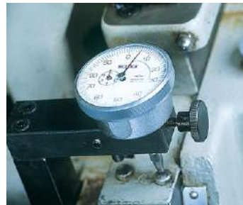
Displacement can be read from above.
