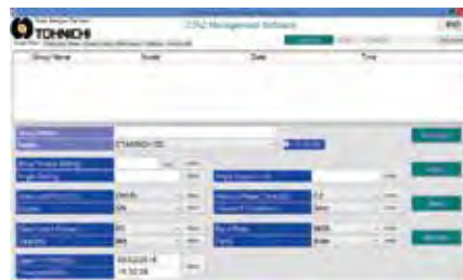
Single spindle tightening mode setting display
